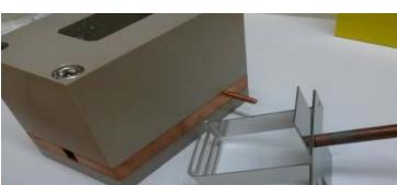
Electrodeposition unit: (left) open showing the stainless steel plate imbedded in the copper cathode; (right) assembled with the platinum anode.
