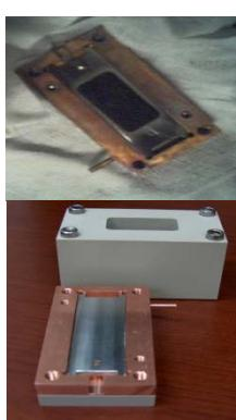
**Figure 2.** (Top) 1.7 Ci Cf-252 electrodeposition inside the hot cell at ORNL's Radiochemical Engineering Development Center
