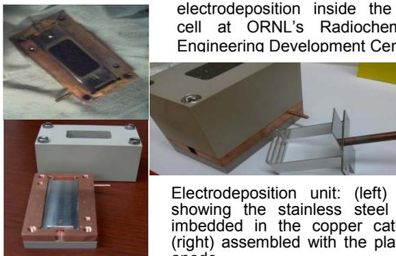
Electrodeposition unit: (left) open showing the stainless steel plate imbedded in the copper cathode; (right) assembled with the platinum anode.
