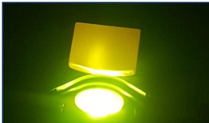
W-182 being heated (round) within the e-beam chamber and specially designed Mo heat shield (rectangle) glowing from secondary electrons (Image courtesy of ORNL)
