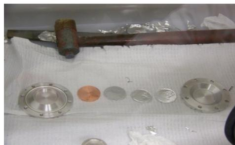
**Actual target components for Ac-225 production – Al shell, 3 Al wrapped Th foils, and Cu disk for energy adjustment.**
