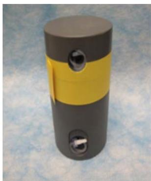
*Radium-224/lead-212 generator as shipped in lead shield (left) and with the shield cap removed to show the tubing connections to the column (right).*
