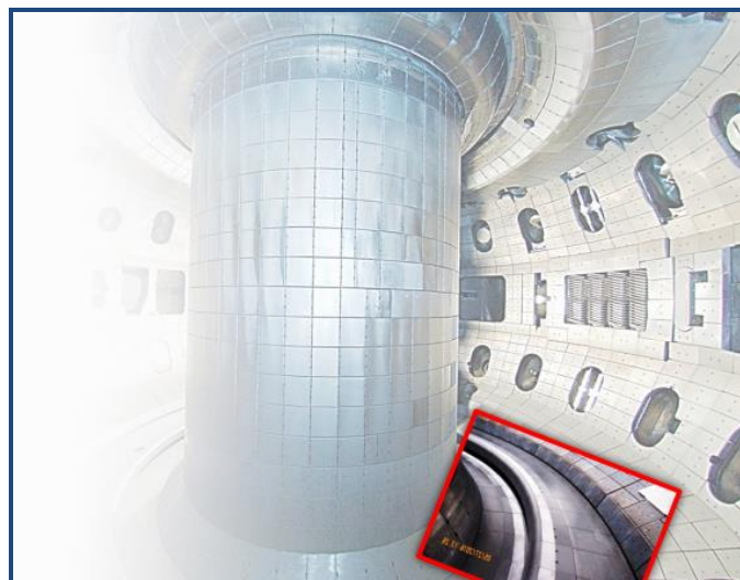
DIII-D tokamak, operated by General Atomics, with natural and W-182 coated molybdenum tiles highlighted in red box (Image courtesy of General Atomics)
