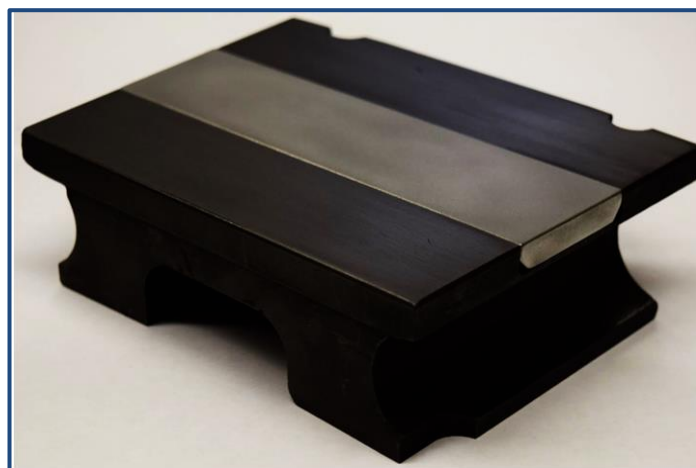
Final resulting W-182 coated molybdenum alloy tile inserted in the DIII-D reactor graphite floor tile before plasma exposure (Image courtesy of ORNL)
