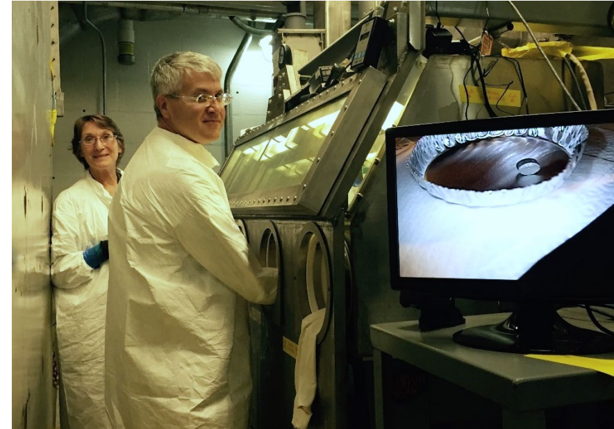
Preparation of ^{226}\text{Ra} targets in a glovebox
